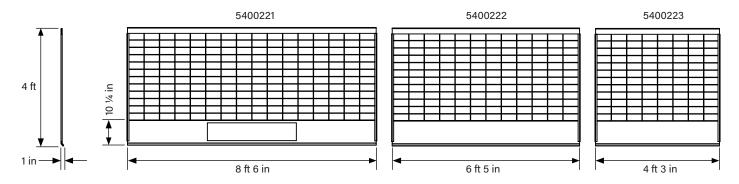
NOTE: There is no minimum amount of overlap required when mounting multiple barriers on a post to create a span. Always ensure barriers are held securely in place by locking mechanism.
