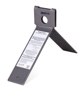
The Snappy Anchor is a one-time-use fall protection anchor designed for combined wood substrates of compatible roof sheathing over trusses. Guardian Fall Protection is clarifying the minimum substrate requirements for the Snappy Anchor. The minimum combined substrate thickness shall be 3½". All fasteners must be fully embedded into truss.
